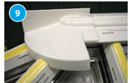
9 Bay and hip-ended lean to roofs require a radius end top cap. This should be sealed and secured to the wallplate top cap with the plastic rivets supplied.
